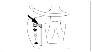
Figure 8. Combined Speed and Choke Control
